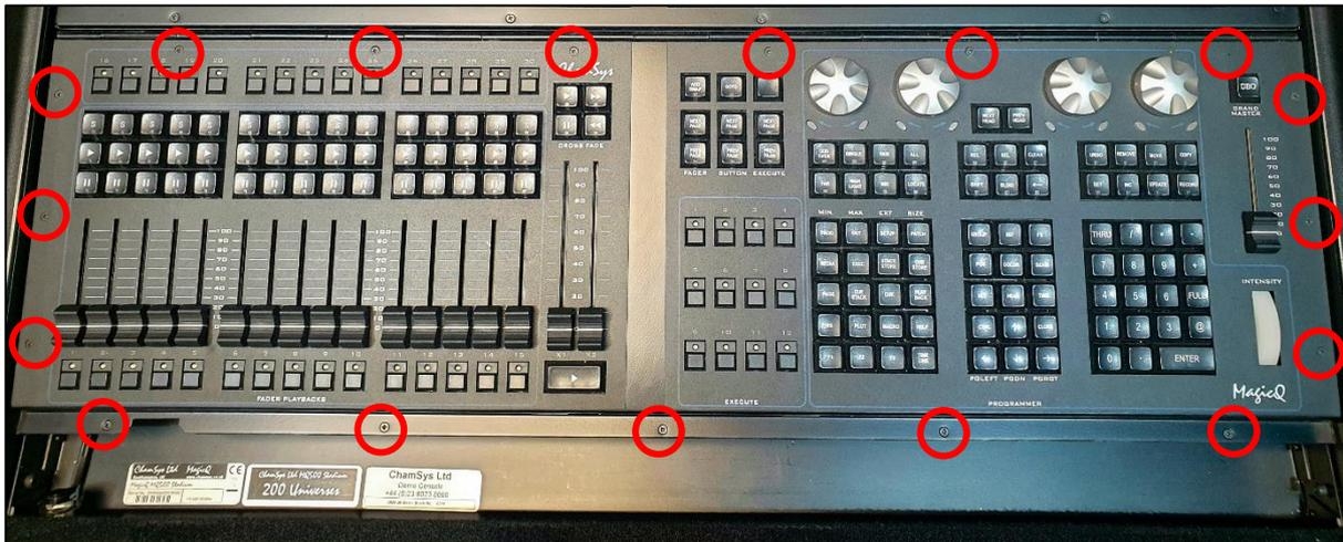
Once all 17 screws have been removed, the front panel assembly can then be lifted carefully from the front. Note that the assembly consists of 2 front panels, and each panel has a cable that must be disconnected to free the assembly completely, as pictured below. Both are locking connectors; push the tab to unlock and pull to release. Once these are disconnected, remove the front panel assembly, and set aside.
