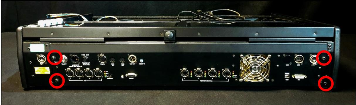
To begin, turn the console around to access the rear and remove the 4x M4 hex screws securing the rear panel in place, using a 4mm ball driver or Allen key. See the image above for screw locations. Once these screws are removed, you can carefully slide the rear panel out, just enough so all components can be accessed as in the image below.
