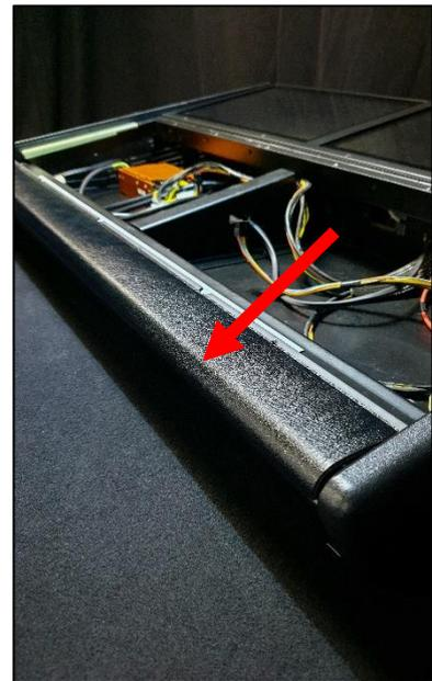
Once in place, screw in the arm rest with 3x M3x6 silver screws. You will find the three screw holes for these just underneath the holes where you previously screwed in the support bracket. Note that while the arm rest is screwed in place, you will need to use some force to pull it towards the front of the console as much as possible. This will not only help line up these screws but is also important when fitting the front panel, ensuring it lines up correctly.
