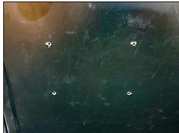
Once the holes are filed and any new metal shavings are removed, you are ready to screw in the new power supply.
